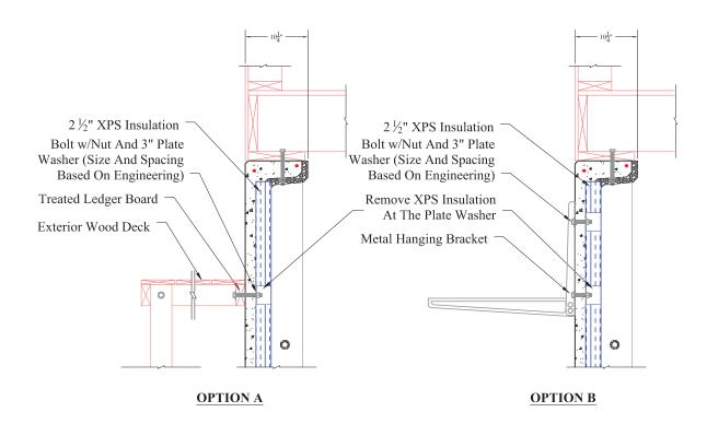
USE POLYURETHANE SEALANT AT BOLT HOLES THROUGH SUPERIOR WALLS PANEL
